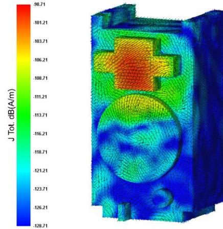
Figure 3. Equivalent electric current on the satellite when the Sarant UHF is fed.
