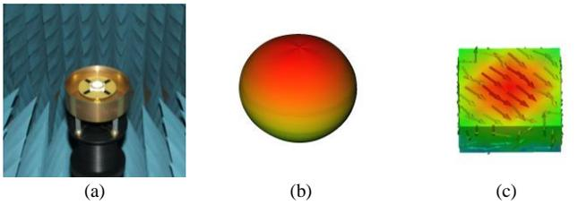
Fig. 2. Source preparation procedure: (a) array single element in the StarLab measurements system; (b) NF radiation pattern @1940MHz; (c) equivalent electric J currents, Huygens box @1940MHz.
