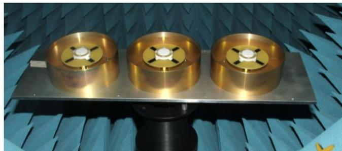
Fig. 1. Linear array of three elements.
