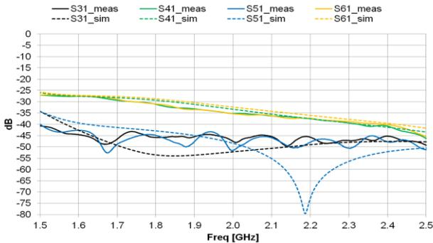
Fig. 4. Antenna coupling between the central element (port 1) and the other two elements (ports 3-6). Comparison between measurement (meas) and simulation using the measured NF model of the central element (sim).
