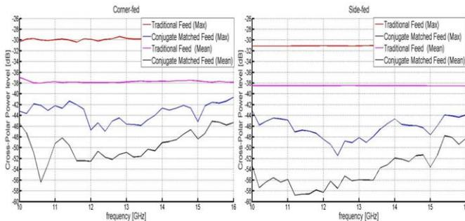
Fig. 3. Maximum and mean QZ cross-polarization normalized to co-polar peak as function of frequency (horizontal polarisation). Proposed feed vs traditional feed. CATR geometry,  $F/D \approx 3$ , 1.7m x 1.7m reflector dimension and serrated edges: Corner-fed (Left), Side-fed (Right).
