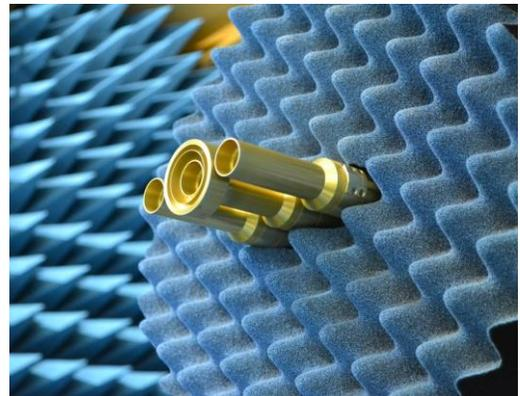
Fig. 1. Conjugate matched feed providing cross-polar 1.6:1 bandwidth in dual linear polarisation.
