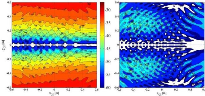
Fig. 2. Contour plots of simulated QZ cross-polarization at 13.0 GHz normalized to co-polar peak (horizontal polarisation). CATR geometry, side-fed,  $F/D \approx 3$ , 1.7m x 1.7m reflector dimension and serrated edges. Standard CATR feed (Left), proposed conjugate matched feed (Right).
