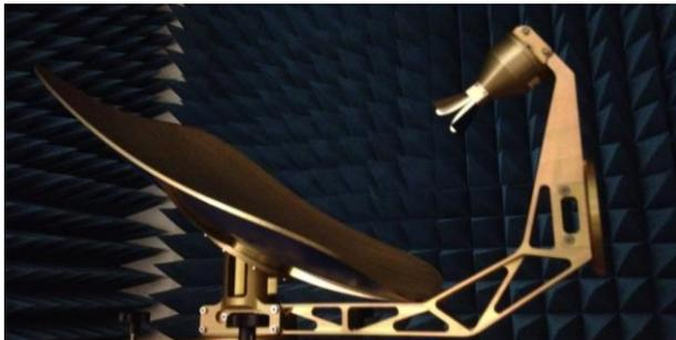
Fig. 1. The reflector antenna used in the validation experiment. SR-40 offset reflector and SH4000 dual ridge horn operating from 4-40 GHz from MVG.
