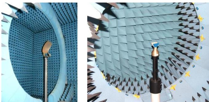
Fig. 2. Reference measurements of the reflector antenna and feed in the MVG SG-64 spherical near field facility in Paris (left). Measurement of the isolated SH4000 dual ridge fed in the MVG StarLab 18 GHz facility in Pomezia, Italy (right).
