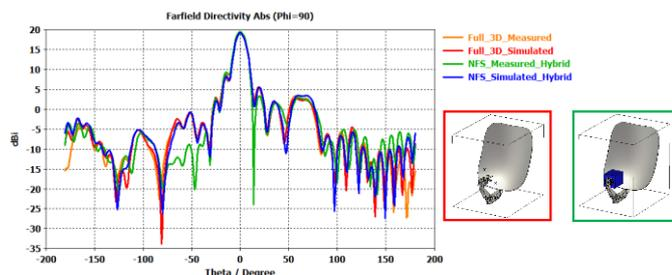
Fig. 3. Elevation plane pattern of the offset reflector antenna feed by the dual ridge horn at 4 GHz. Results from the proposed method combining measured feed pattern and numerical modelling, compared with direct measurement and full numerical modelling.
