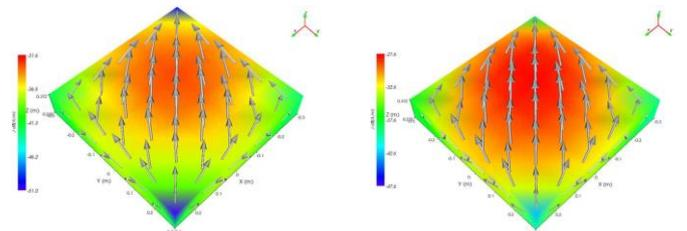
Fig. 4. Equivalent electric currents of the stand alone elements with solid (Left) and slotted (Right) ground plane.
