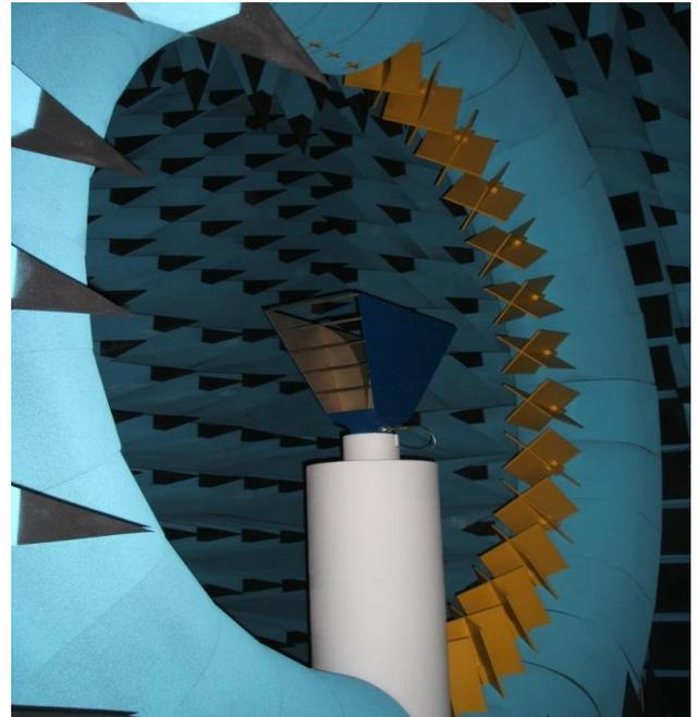
Fig. 1. Example of spherical multi-probe system.
