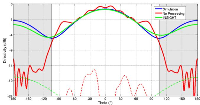
Fig 5. E-plane directivity pattern comparison of the stand alone solid ground plane element.
