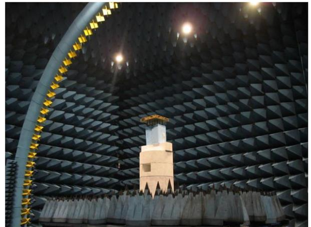
Fig. 3. AIS antenna in the embedded configuration during measurement in hemispherical range.
