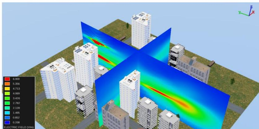
In addition, the new version allows users to assign material properties to the entire surrounding 3D environment in order to take into account their impact on exposure levels and still makes fast calculations.
