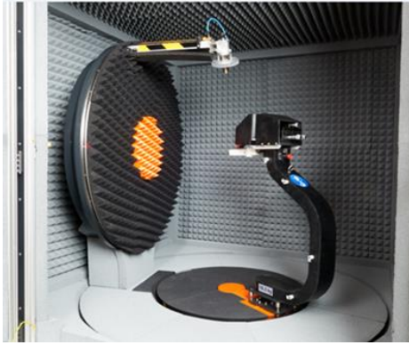
Fig 4. Orbit/FR \mu Lab on-chip measurement setup
