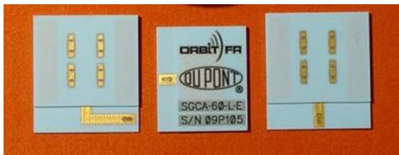
**Figure 2:** Photo showing three feed orientations for the 60GHz reference antenna. From left to right: i) zenith radiating with feed orthogonal to H-Plane, ii) nadir radiating with feed orthogonal to E-Plane, and, iii) zenith Radiating with feed orthogonal to E-plane.
