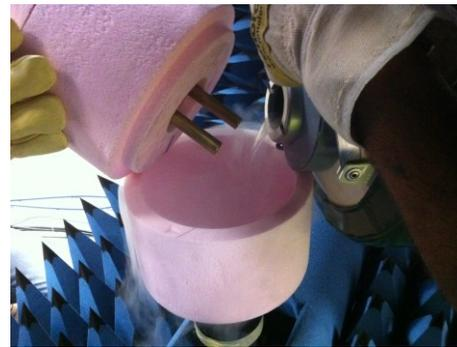
Figure 13. Pouring of the nitrogen in the climate box. The heat transfer is primarily provided by the immersion chiller shown.
