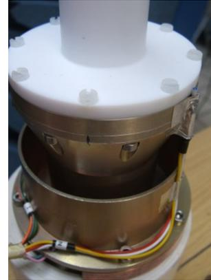
Figure 9. Detail of the AUT. RFD thermistors have been placed around the AUT ground plane.
