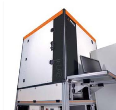
Figure 1. : MVG  $\mu$ -Lab: millimeter wave Spherical Near-Field measurement system.
