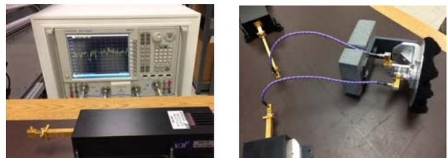
Figure 13. : Test set-up for S-parameters: reflection coefficients (left), port-to-port isolation (right).
