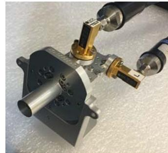
Figure 11. : MVG SP50000 probe (w/o absorber screen).
