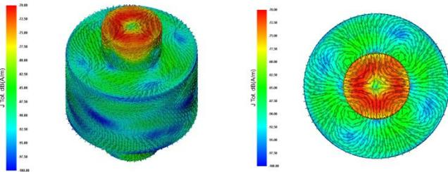
Fig. 3. Equivalent Currents @ 1250MHz associated to  $|\mu| = 2$  spherical modes only. 3D-view (left); top-view (right).
