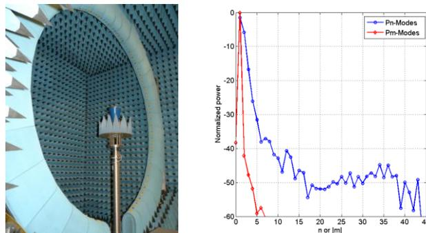
Fig. 1. MVI SP1100 probe during calibration in SNF in MVG SG64 (left); Measured spherical mode spectrum @ 1.25 GHz (right).
