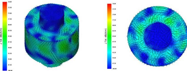
Fig. 4. Equivalent Currents @ 1250MHz associated to  $|\mu| > 2$  spherical modes only. 3D-view (left); top-view (right).
