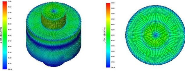
Fig. 2. Equivalent Currents @ 1250MHz associated to  $\mu = 0$  spherical modes only. 3D-view (left); top-view (right).
