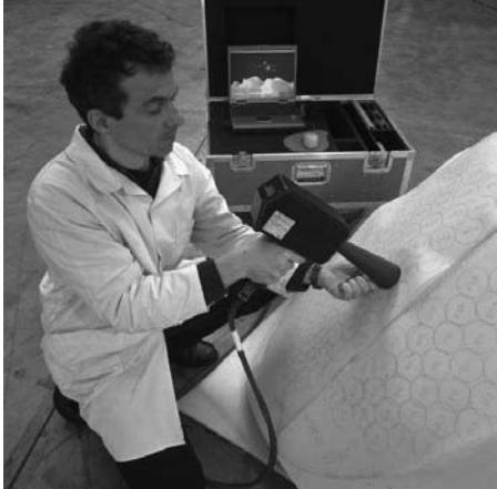
Figure 2. Use of a portable device for the diagnosis of radomes in repair shop [5].
