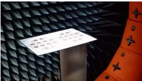
Fig. 3. : Patch antenna in the StarLab18GHz measurement system [4]. Only one of the separate arrays is measured.
