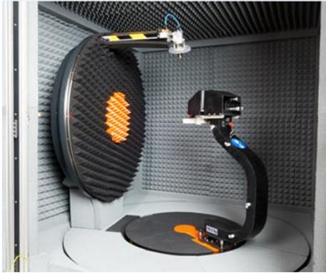
Fig 4. Orbit/FR  $\mu$ Lab on-chip measurement setup
