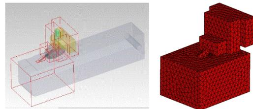
Fig 3. AUT and the measurement set-up, showing reconstruction geometry (left); meshed reconstruction geometry (right).
