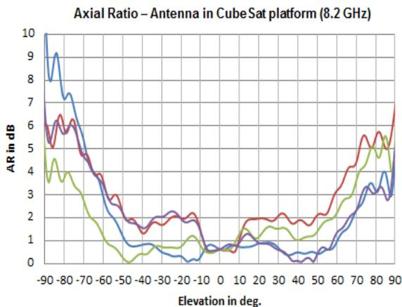
Fig. 10: Measured axial ratio (8.2 GHz)
