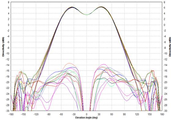
Fig. 5: Simulated radiation pattern (8.2 GHz)
