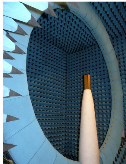
Fig. 8: Measurement of the antenna in the SG-64 facility
