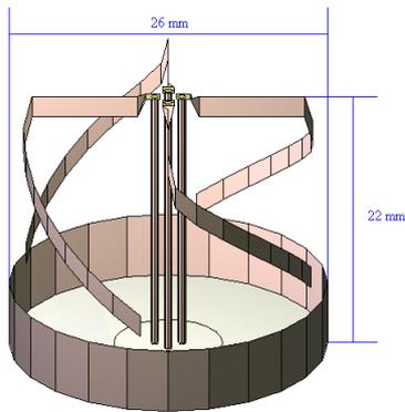
Fig. 2: Miniaturized quadrifilar wire helix antenna
