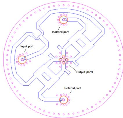
Fig. 4: Antenna feeding circuit
