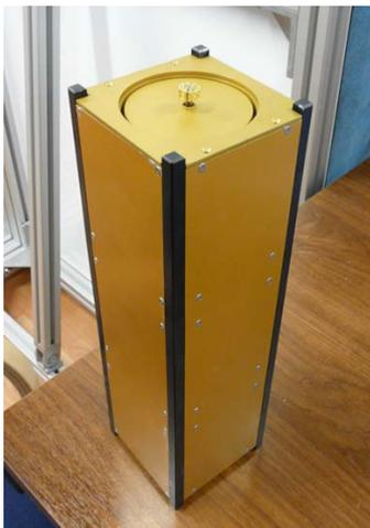
Fig. 6: Manufactured CubeSat 3U platform with antenna on top
