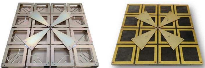
Figure 1. AISMAN engineering models: metallic (left); composite material (right).
