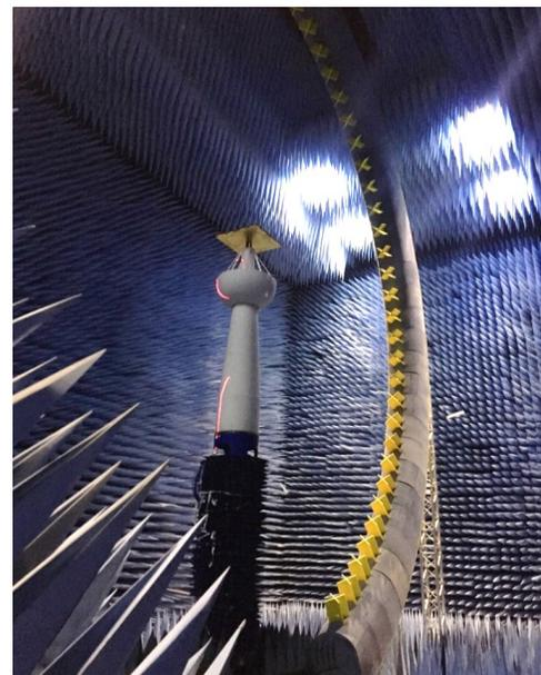
Figure 7. Improved AIS element during measurement in CAST 501 spherical multi-probe range (courtesy of CAST 501).
