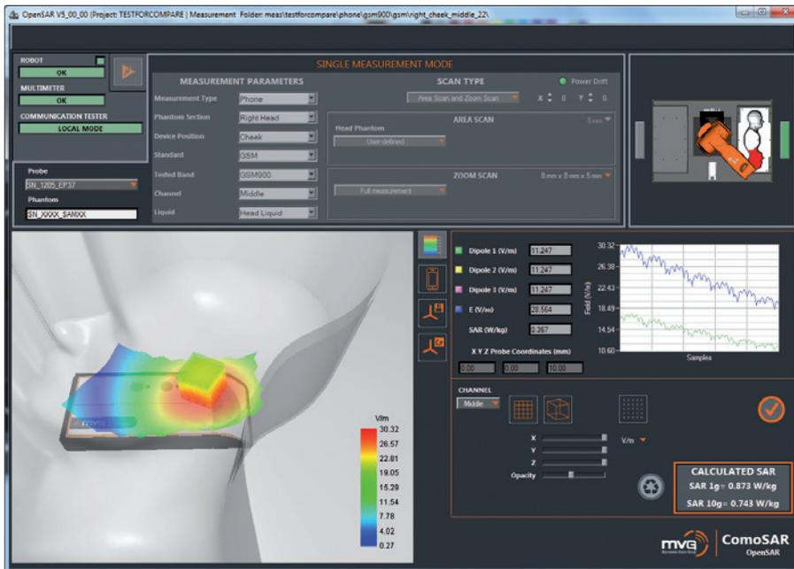
OPENSAR software has been developed to perform SAR standard compliant measurements. It is part of MVG's COMOSAR bench and controls all the instrumentation delivered with this bench.
