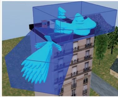
EMF Visual integrates a Massive MIMO antenna database with 2D array antennas working at 3.5GHz, 28GHz, 39GHz together with a dedicated function for adjusting easily the beam steering range in azimuth and elevation.
