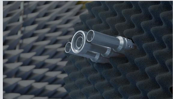
In the most common compact range reflector systems, a large reflector is illuminated by a feed to ensure that the amplitude and phase variation is minimal across the Quiet Zone (QZ). To avoid obstruction by the feed an offset reflector geometry is used. This offset geometry causes a cross-polarization as a function of position in the QZ.
