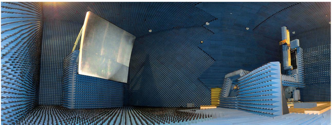
Compact range with a rolled-edge reflector
