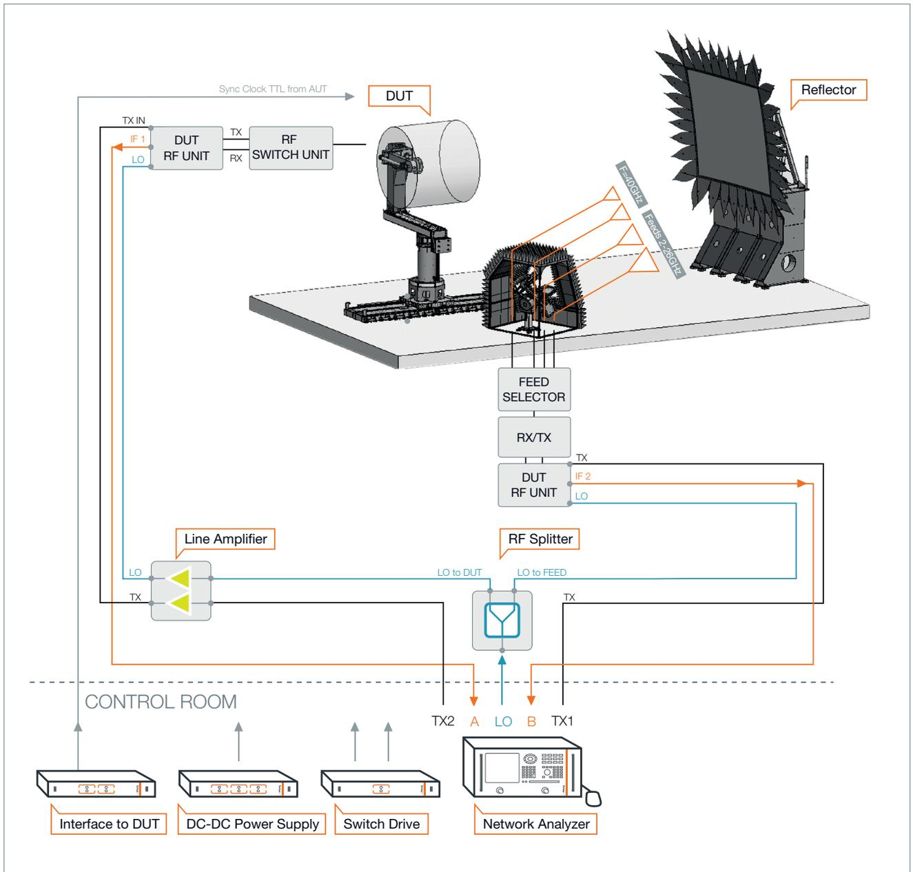
The lowest operational frequency of a compact range system is determined by the size of the reflector, the edge treatment and the absorbers.
