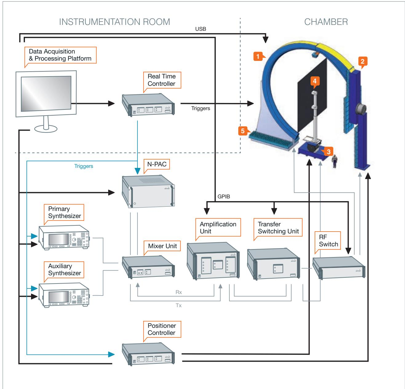
G-DualScan uses a Vector Network Analyzer as the RF source/receiver for antenna measurements. The Amplification Unit has RF amplifiers for each of the RX and TX channels. G-DualScan uses a Transfer Switching Unit to emit from the AUT to the probe(s) or vice versa. A dedicated RF switch allows the selection of either the single-probe or the multi-probe set-up. The Positioner
