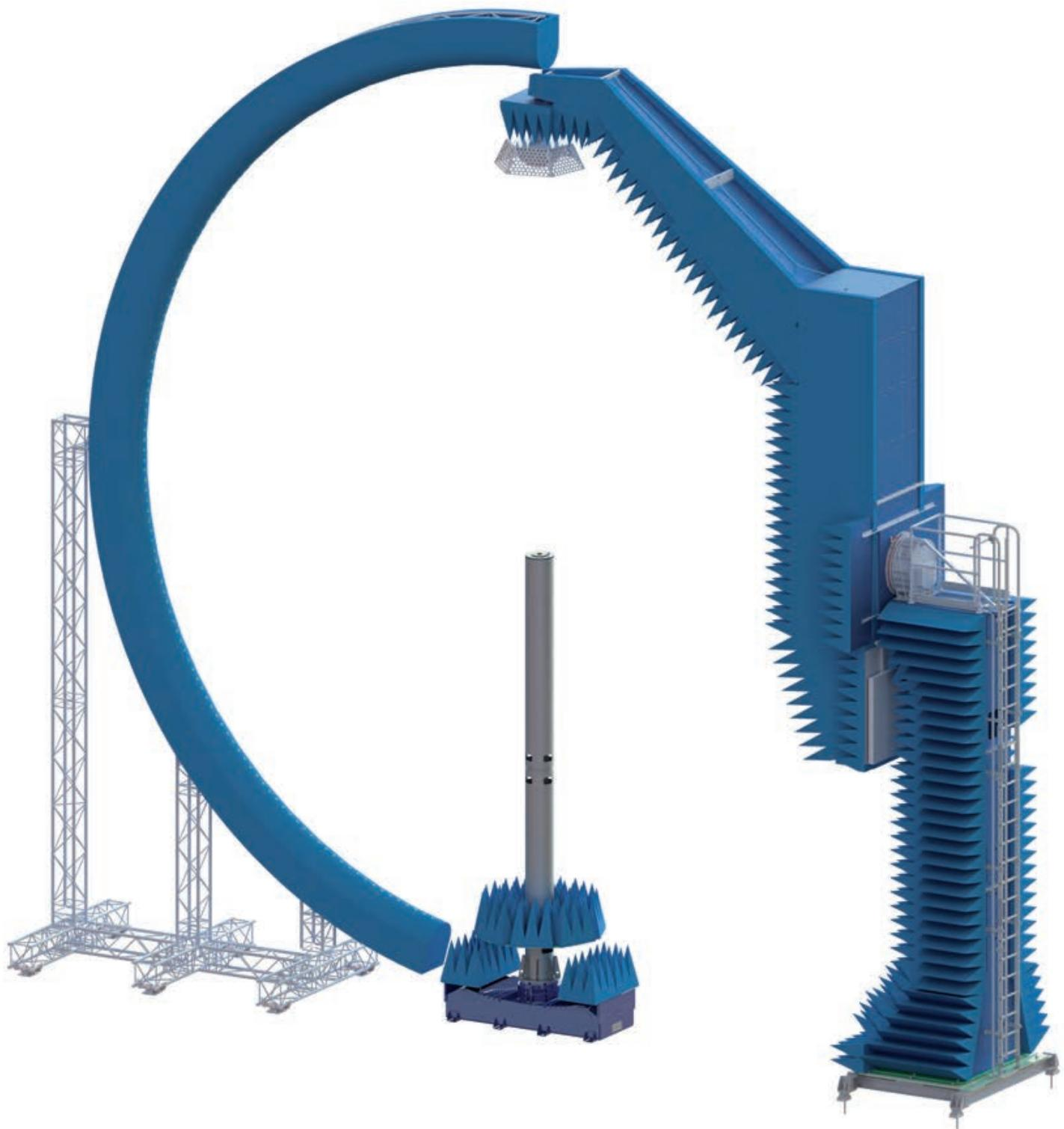
G-DualScan represents a step forward in spherical near-field measurements. It measures antennas with large dimensions and analyzes a very broad range of frequency bands from 200 MHz to 18 GHz. It consists of a single-probe gantry arm and a multi-probe arch up to 12 meters (40 feet) in diameter.
