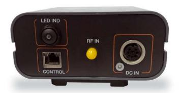
Solid state absorptive polarization PIN switches are an optimal solution to operate dual polarized antennas. They are suitable for use with compact range feed antennas and for near field probes. Covering a wide frequency range, up to 50 GHz at a switching time of 50 nsec, these switching units work well with systems which combine low and high-power antenna measurement (with high power attenuator according to customer request).
