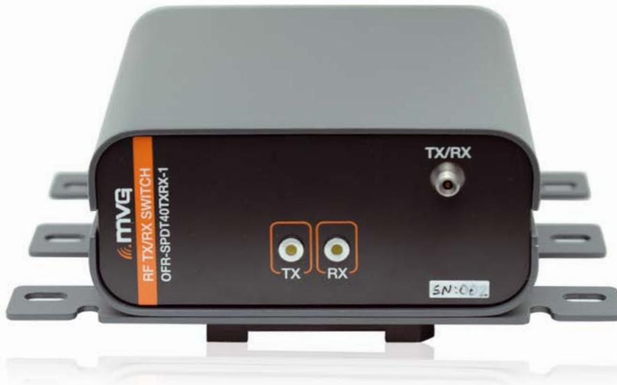
50-ohm coaxial switches are designed to toggle between TX and RX operational modes. These RF units are designed to handle power levels up to 80 W at a switching time of 10 ms (milliseconds). The RF signals can be amplified with an internal broadband LNA.
