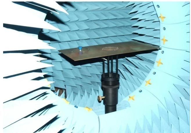
Fig. 1. Validation structure during measurement in the MVG Spherical Near Field antenna measurement system, StarLab18GHz [16].
