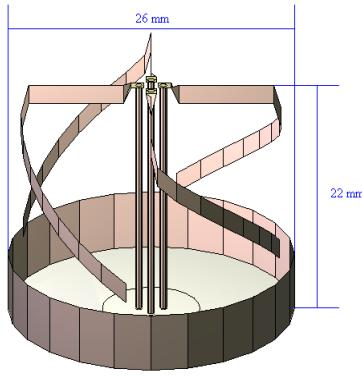
Fig. 2: Miniaturized quadrifilar wire helix antenna
