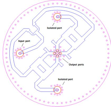
Fig. 4: Antenna feeding circuit
