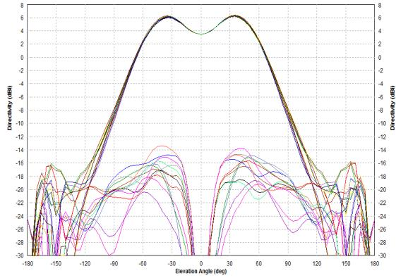
**Fig. 5: Simulated radiation pattern (8.2 GHz)**
