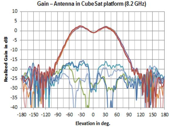
Fig. 9: Measured gain radiation pattern (8.2 GHz)
