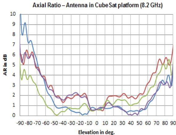
Fig. 10: Measured axial ratio (8.2 GHz)
