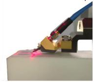
**Figure 9:** Picture of microprobe landing on the 60GHz reference antenna that has been placed on a low density chuck.
