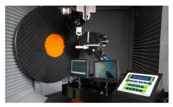
**Figure 8:** Photo of the chamber interior with the vision system and real-time S11 feedback to assist probe landing.
