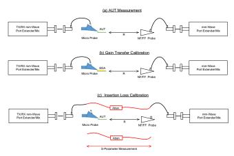
Figure 11: Simplified System Diagram for (a) AUT (Chip) Measurements, (b) Gain Transfer Method using onchip gain standard, and (c.) Insertion Loss Method Calibration including the direct cable/attenuator S21 measurement.
