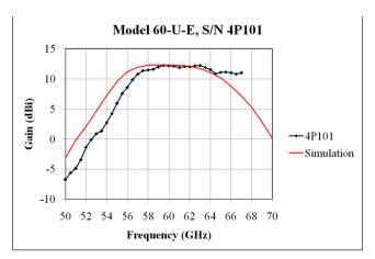
Figure 4: S/N 4P101 Peak Gain vs. Frequency
