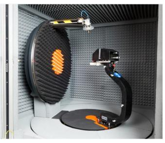
Figure 7:Photo of interior of the  $\mu$ -lab test system configured micro-probing
