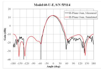
Figure 6: S/N 5P114 H-Plane Gain vs. Angle
