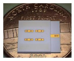
Figure 1: 60GHz 2x2 array chip antenna placed on a US Quarter
