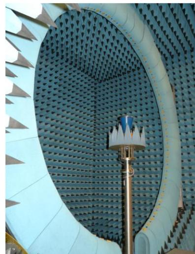
Fig. 2. MVI SP1100 probe during SNF measurement in MVG SG64 spherical multi-probe system.
