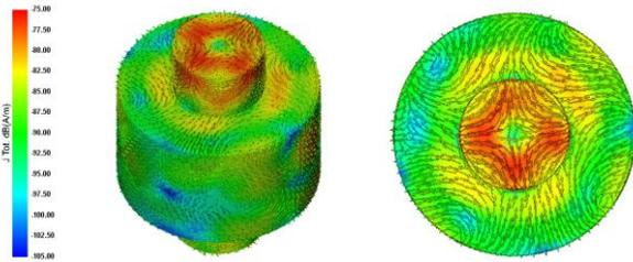
Fig. 7. Equivalent Currents @ 1250MHz associated to  $|\mu| > 1$  spherical modes only. 3D-view (left); top-view (right).
