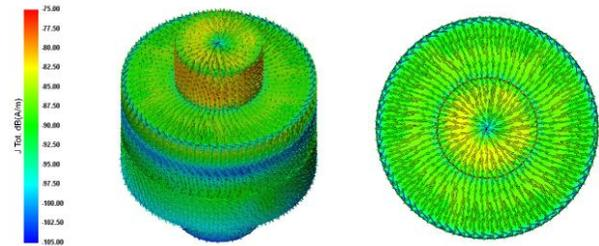
Fig. 6. Equivalent Currents @ 1250MHz associated to  $\mu = 0$  spherical modes only. 3D-view (left); top-view (right).
