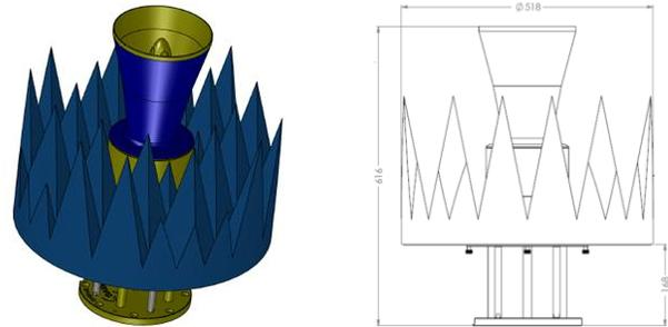
Fig. 1. CAD model of the MVI SP1100 probe.
