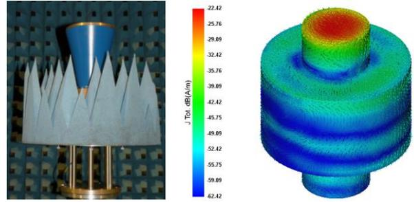
Fig. 5. Equivalent electric currents @ 1250MHz evaluated on an equivalent geometry encompassing the MVI SP1100 probe.
