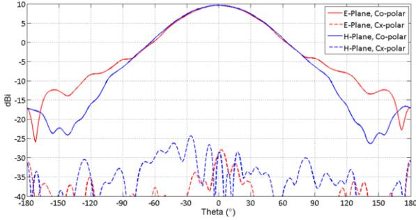
Fig. 3. Measured directivity pattern of the MVI SP1100 probe @ 1250MHz. E-plane pattern cut (red traces); H-plane pattern cut (blue traces).
