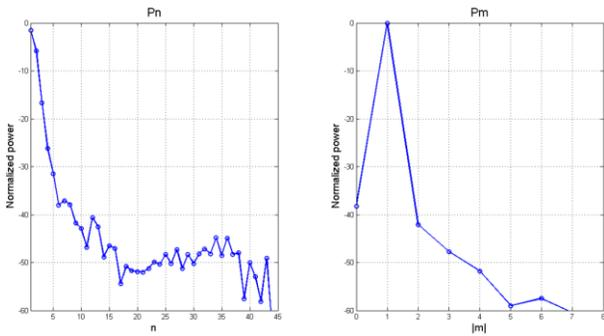
Fig. 4. Measured spherical mode spectrum @ 1250MHz of the MVI SP1100 probe.  $P_n$ -modes (left);  $P_m$ -modes (right).
