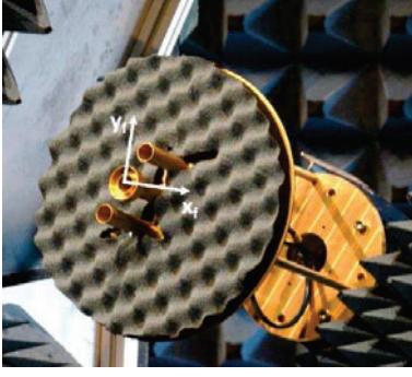
Figure 1. The proof-of-concept demonstrator configured for a corner-fed single CATR
