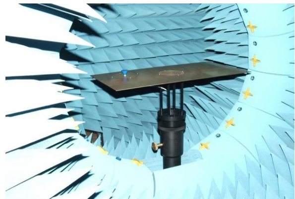
Fig. 1. Validation structure measured in the Spherical Near Field antenna measurement system, StarLab18GHz [10].
