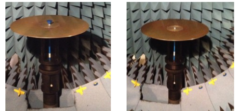
Fig. 4. Measurement of the monocone antenna, monopole antenna on a limited ground plane in the MVG, SL18GHz spherical near-field multi probe system [14].
