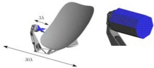
Figure 2. Example of reflector antenna where the feed (in blue, on the left) is enclosed in a surface (in blue, on the right) to generate the basis functions.
