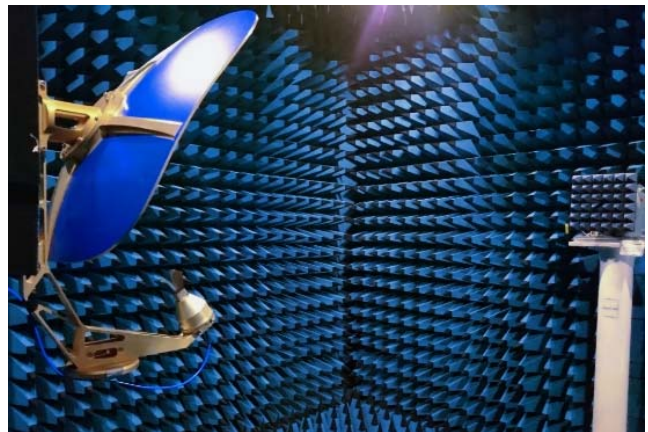
Figure 3. MVG SR40-A fed by a SH4000 dual-ridge horn in the SNF range at Politecnico di Torino.
