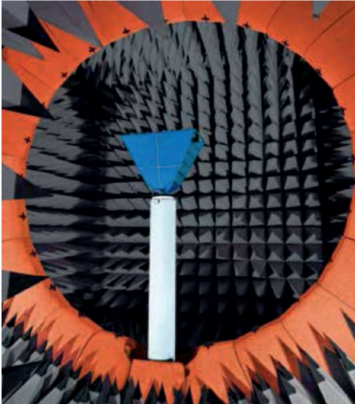
Figure 2: Measurement of a horn antenna, using MVG StarLab measurement system.
