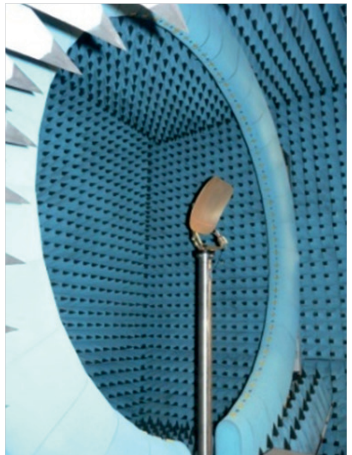
Figure 8: Reference measurements of the reflector antenna and feed in the MVG SG-64 spherical nearfield facility in Paris.
