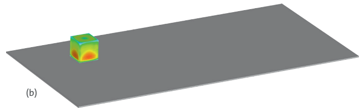
Figure 12: SMC2200 monocone antenna flushed mounted on the plate (a) and the equivalent model in CST STUDIO SUITE with the measured Nearfield source (b).
