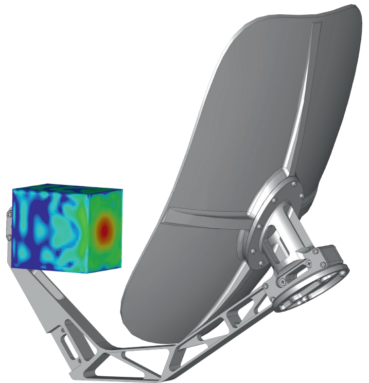
Figure 6: Nearfield source imported in CST STUDIO SUITE and mounted on the reflector dish CAD model.
