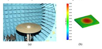
Fig. 2. Source preparation procedure: (a) OEW on a cirucal ground pèlane in the StarLab measurements system (c) equivalent electric J currents, Huygens box @4380MHz.
