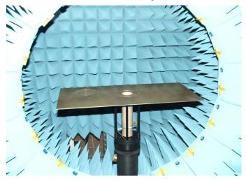
Fig. 1. Validation structure during measurement in the Spherical Near Field antenna measurement system, StarLab18GHz [10].
