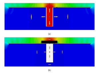
Fig. 4. OEW on the ground plane, E near field comparison at x=0mm @4380MHz [5]. (Up) Measured source (EQC) (black box); (Bottom) Full wave simulation. Upper face of the ground plane is center with respect to the xy plane and placed at z=0mm. The dynamic range is 40dB.
