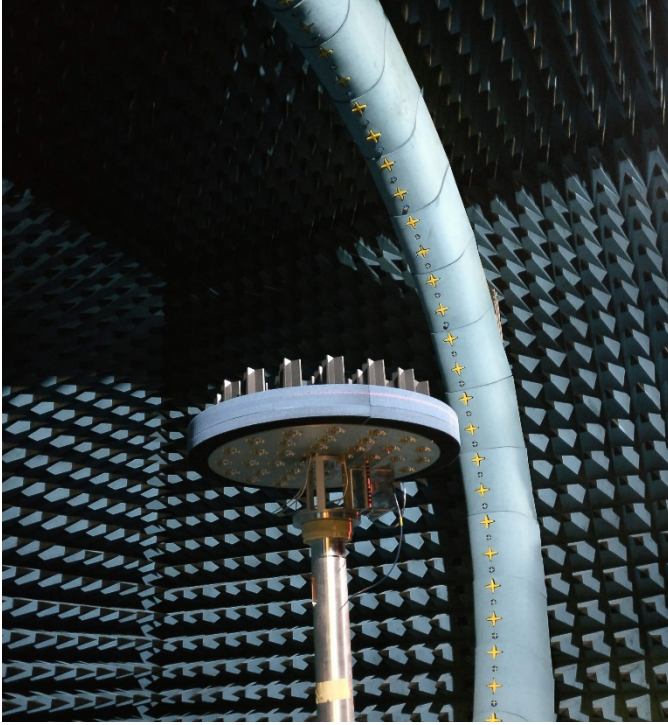
Figure 2. PWG during validation measurement in the spherical NF multi probe system SG-64 in Paris.
