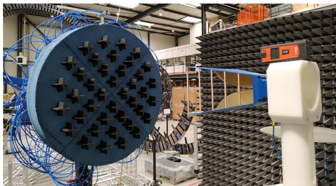
Figure 5. Illustration of the on-axis gain measurements using the PWG prototype. The antenna and reference antenna are placed in different positions within the QZ.
