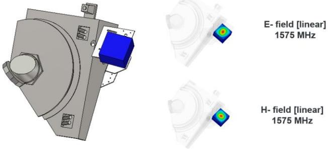
Figure 8. Placement and simulation in CEM tool @ 1575MHz.
