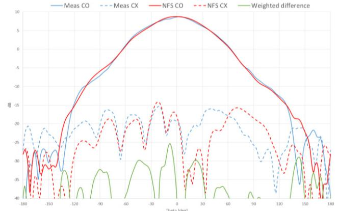
Figure 9. Copolar and crosspolar components at phi=0° of measurements (MEAS) and of CST simulation based on INSIGHT NF measured Source (NFS) at 1227 MHz.
