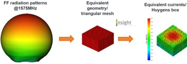
Figure 6. Antenna characterization in terms of EQC using INSIGHT @ 1575MHz.
