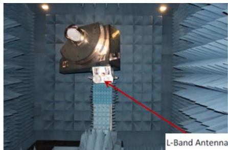
Figure 2. Sentinel satellite mock-up (RUAG courtesy).
