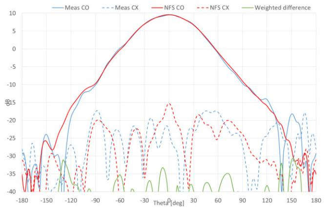
Figure 11. Copolar and Crosspolar components at phi=0° of measurements (MEAS) and of CST simulation based on INSIGHT NF measured Source (NFS) at 1575 MHz.
