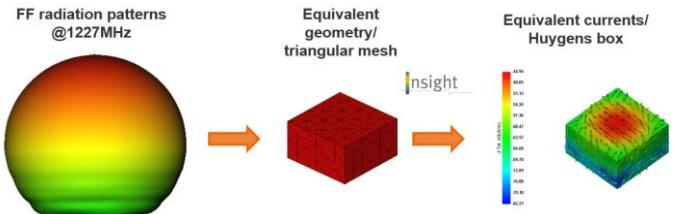
Figure 5. Antenna characterization in terms of EQC using INSIGHT @ 1227MHz.
