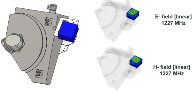
Figure 7. Placement and simulation in CEM tool @ 1227MHz.
