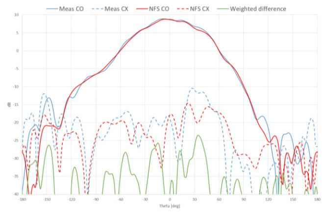
Figure 10. Copolar and Crosspolar components at phi=90° of measurements (MEAS) and of CST simulation based on INSIGHT NF measured Source (NFS) at 1227 MHz.
