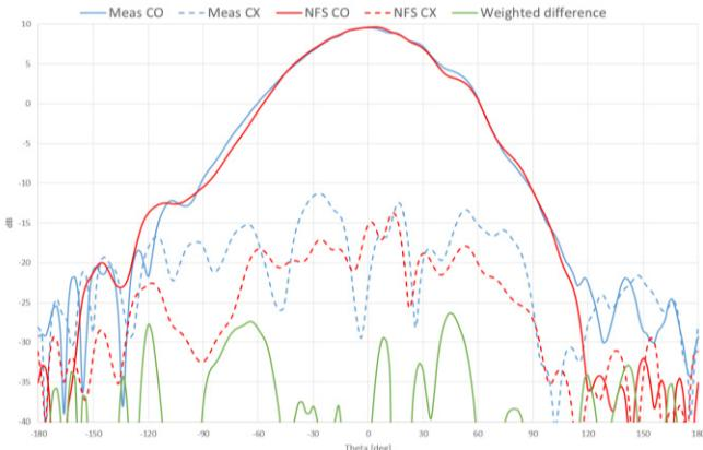
Figure 12. Copolar and Crosspolar components at  $\phi=90^\circ$  of measurements (MEAS) and of CST simulation based on INSIGHT NF measured Source (NFS) at 1575 MHz.
