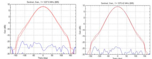
Figure 4. Gain pattern of the GNSS antenna at 1227 MHz (left) and 1575 MHz (right).
