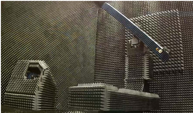
Fig. 8. Field probe scanner mounted on the DUT positioner at diagonal -45 degree.
