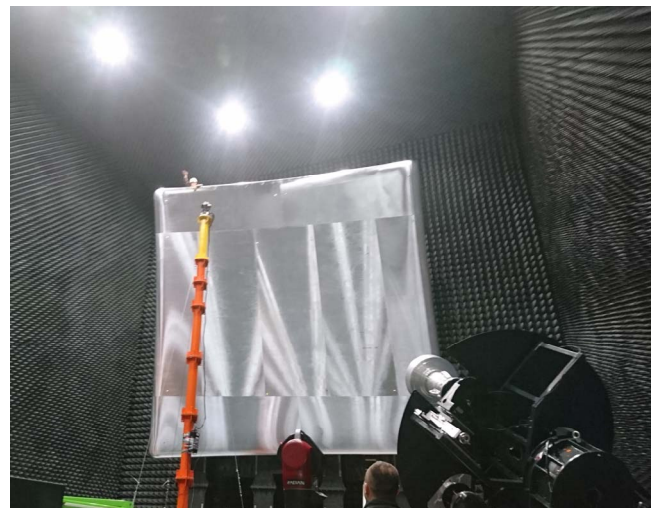
Fig. 2. Photo from the laser tracker alignment of the reflector segments.
