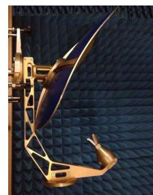
Figure 1. Reflector SR 40-A fed by SH4000 Dual Ridge Horn: Antenna during measurement
