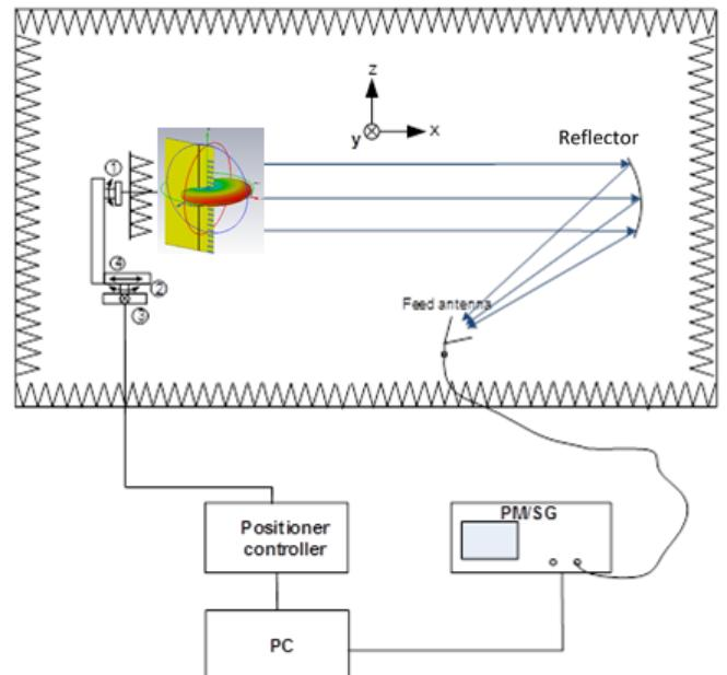
Fig. 9. Typical CATR set up for EIRP measurements
