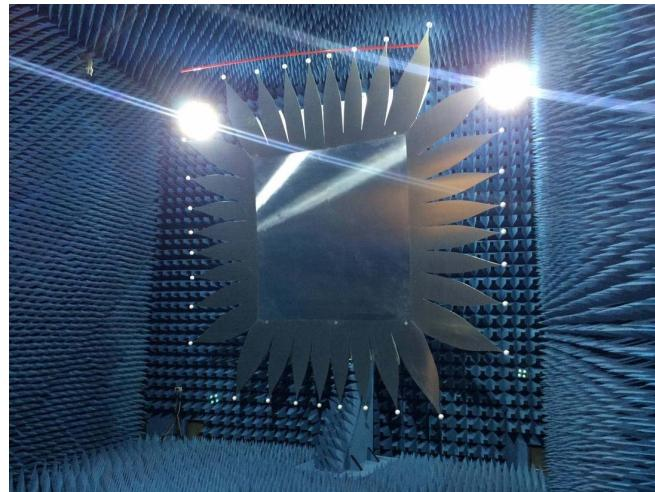
Fig. 1. Serrated-edge reflector
