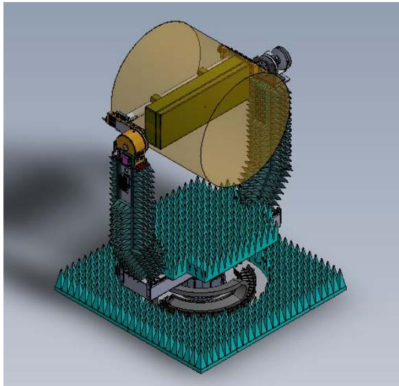
Fig. 3. El/Az positioner for AAS-BS – The Quiet Zone volume is represented by the light yellow cylinder
