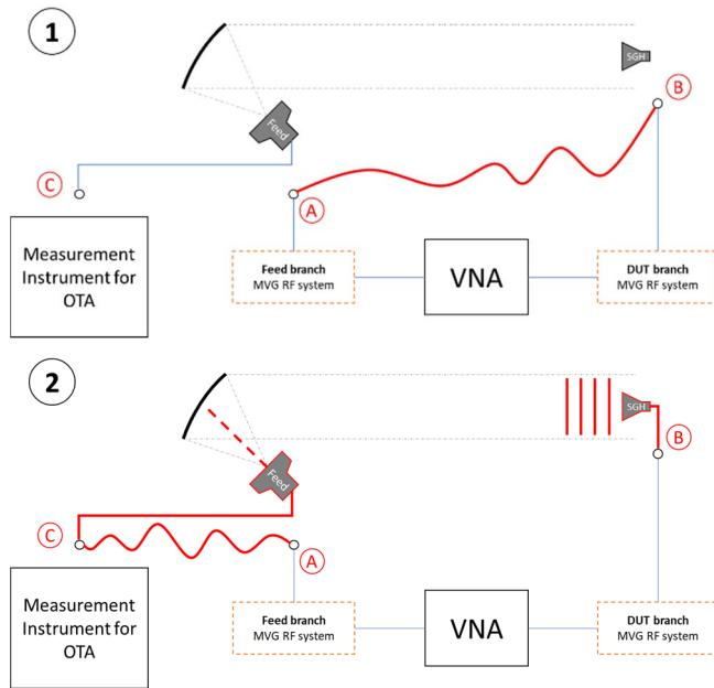
Fig. 8. OTA path loss calibration procedure – the path measured in each calibration step is in red color
