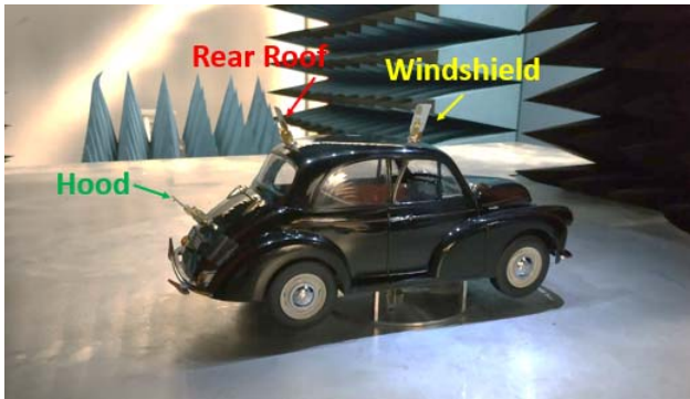
Fig. 3. Scaled vehicle with patch antennas in three different positions.
