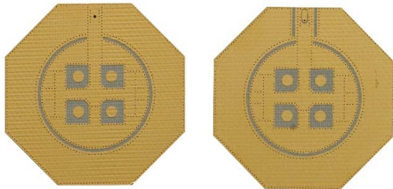
Figure 1. Reference Chip Antennas in Nadir (left) and Zenith (right) configuration.
