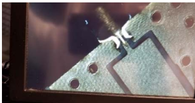
Figure 3. Microscope view of the landed micro-probe tip.
