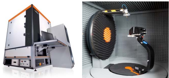
Figure 4. \mu -Lab: mm-wave Spherical Near-Field measurement facility.
