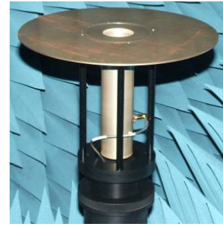
Figure 7: Truncated circular waveguide with finite size ground plane. D=0.3\text{m}/0.6\text{m} @ 4.38\text{GHz} ( 4.4\lambda and 8.8\lambda roughly).
