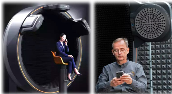
Figure 3. Plane Wave Generator systems for millimeter-wave applications in personal communication [9].
