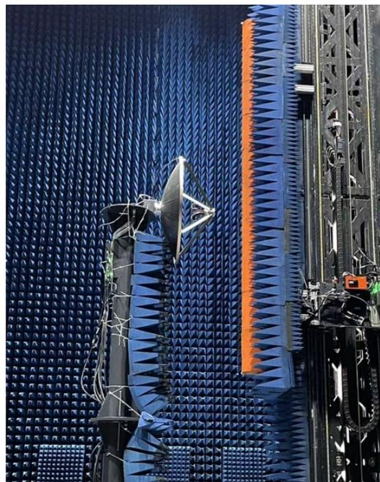
Figure 1. Linear multi-probe array measuring the SR150 onset reflector antenna.
