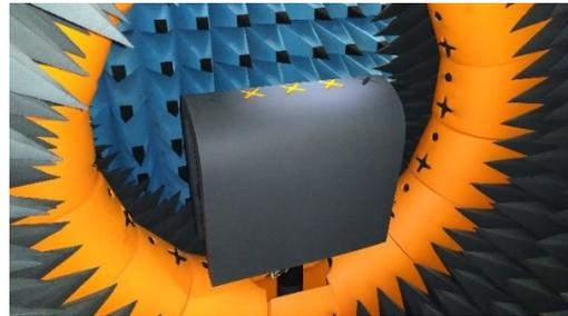
Figure 2. 3-element linear array mock-up during measurement in the StarLab spherical NF system.
