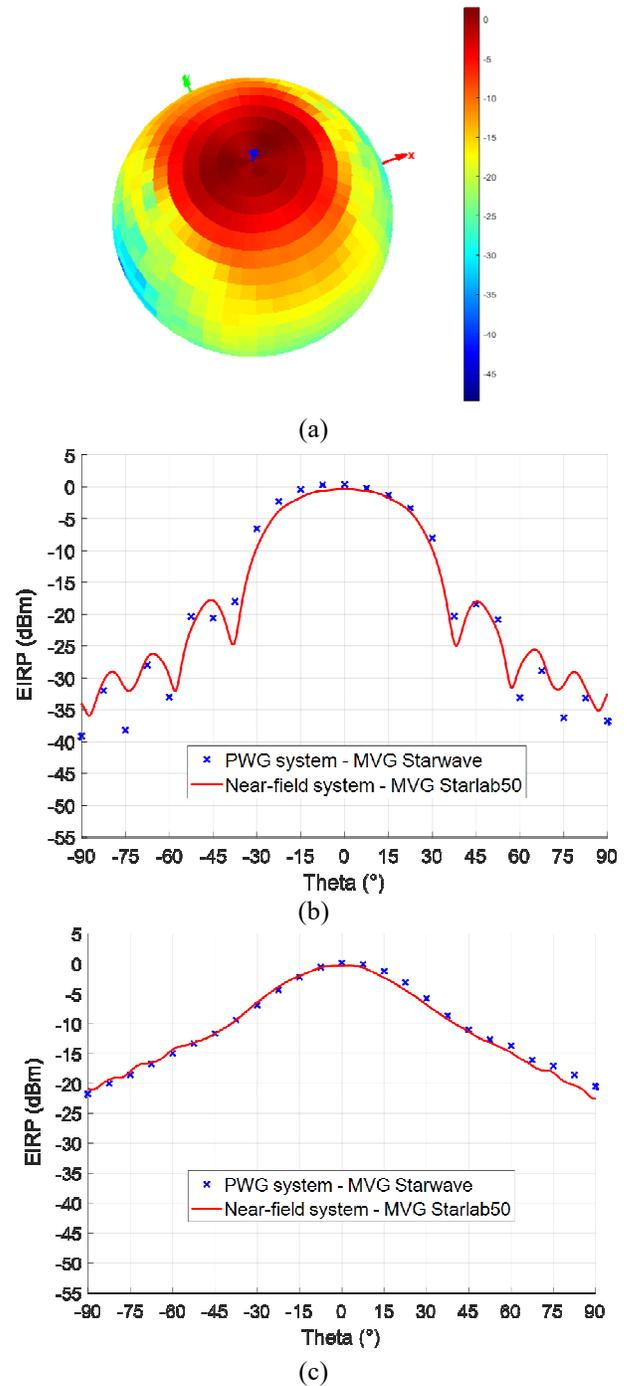
Figure 2. (a) 3D EIRP of SH5000 horn measured in PWG based MVG Starwave system at 28GHz, (b) E-plane, and (c) H-plane EIRP curves comparison between PWG based MVG Starwave and Multi-probe Near-field MVG Starlab50 system at 28GHz
