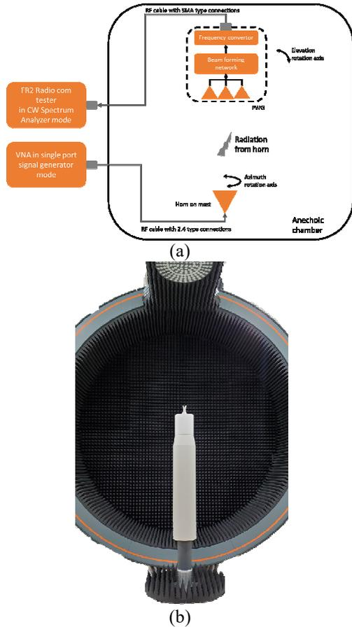
Figure 1. Active measurement setup, (a) block diagram, (b) measurement system picture
