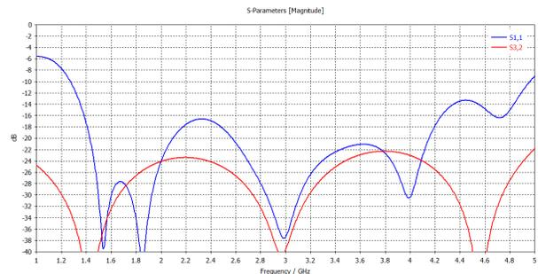
Figure 15. Matching and output ports isolation of the coupler.
