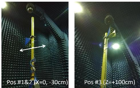
Figure 23. Test campaign in SNF with offset AUT (SH400).
