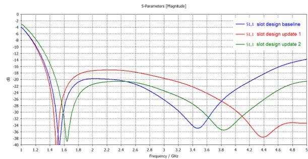
Figure 9. Matching optimization of the slot coupler versus the layout of the slot.
