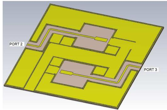
Figure 13. View of the upper face of the printed circuit of the complete coupler.
