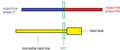
Figure 4. Schematic of the architecture of a coupler based on a common slot coupling.
