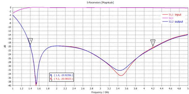
Figure 8. S-parameters of the slot coupler enclosed in its metallic cavity.
