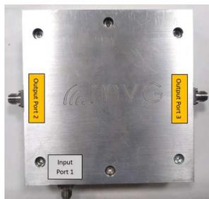
Figure 18. Manufactured coupler covering 1.4-4.2 GHz nominal band.
