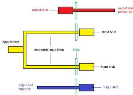
Figure 3. Schematic of the architecture of a coupler based on two separated slot couplings.
