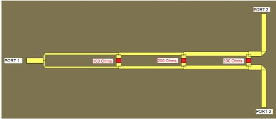
Figure 10. Layout of the three sections Wilkinson divider.
