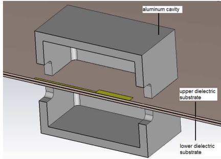
Figure 6. Side cut view of the slot coupler enclosed in its metallic cavity.
