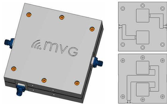
Figure 14. CAD view of the cased 3dB/180° coupler (left), view of the inner layout of the aluminum shells (right).
