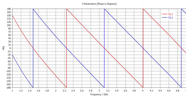
Figure 17. Phase distribution over the output ports of the coupler (0.5° max deviation in nominal band).
