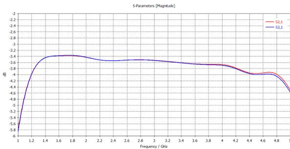
Figure 16. Amplitude distribution over the output ports of the coupler (0.02 dB max deviation in nominal band).
