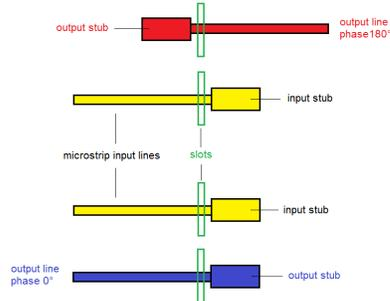
Figure 2. Description of the  $180^\circ$  phase reversal mechanism obtained thanks to slot coupling between microstrip lines.
