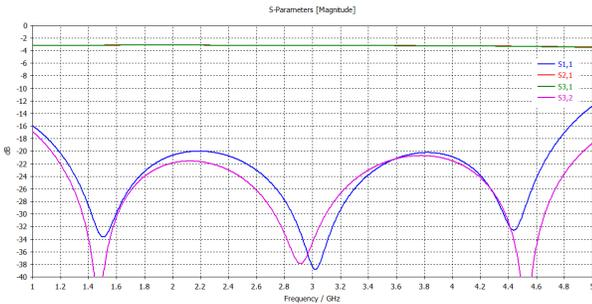
Figure 11. S-parameters of the three sections printed Wilkinson divider.
