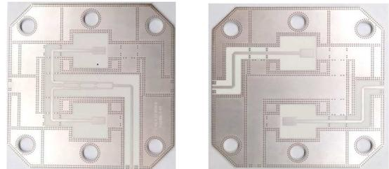
Figure 19. Printed circuit board: lower face (left) and top face (right).
