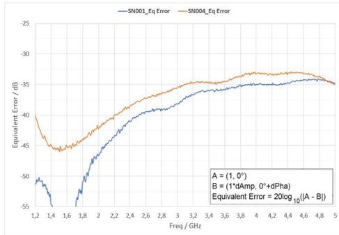
Figure 22. Equivalent error of the manufactured couplers.
