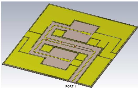
Figure 12. View of the lower face of the printed circuit of the complete coupler.
