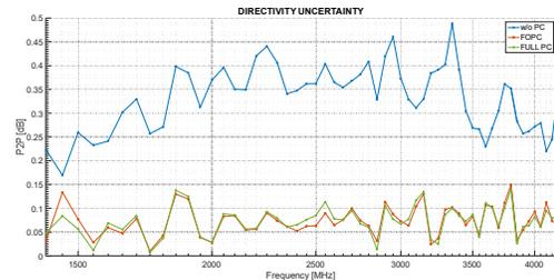
Figure 24. Max directivity variation of the SH400 measured in three different positions and different levels of PC.
