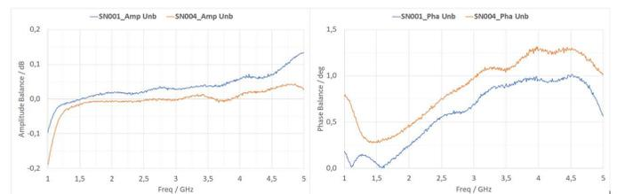
Figure 21. Unbalance between output ports: amplitude (left) and phase (right).
