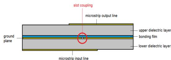
Figure 1. Description of the slot coupling mechanism between two microstrip lines.
