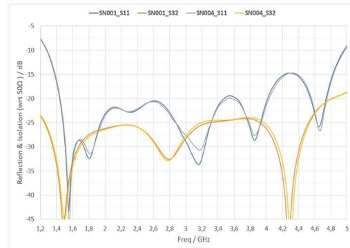
Figure 20. Input reflection coefficient and isolation between output ports (referenced to 50 Ω).
