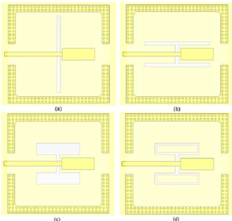
Figure 7. Evolution of the slot layout to improve performance (matching and bandwidth).
