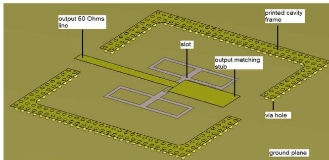
Figure 5. Metallic printed structure of a slot coupler.
