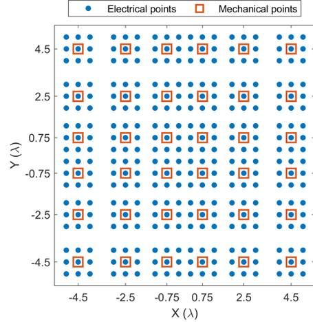
Fig. 2. Example of PWM illustrating the concept of mechanical and electrical measurement points
