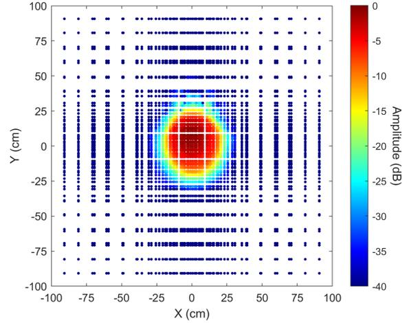
Fig. 6. Electrical points coordinates of the optimized PWM and near-field.
