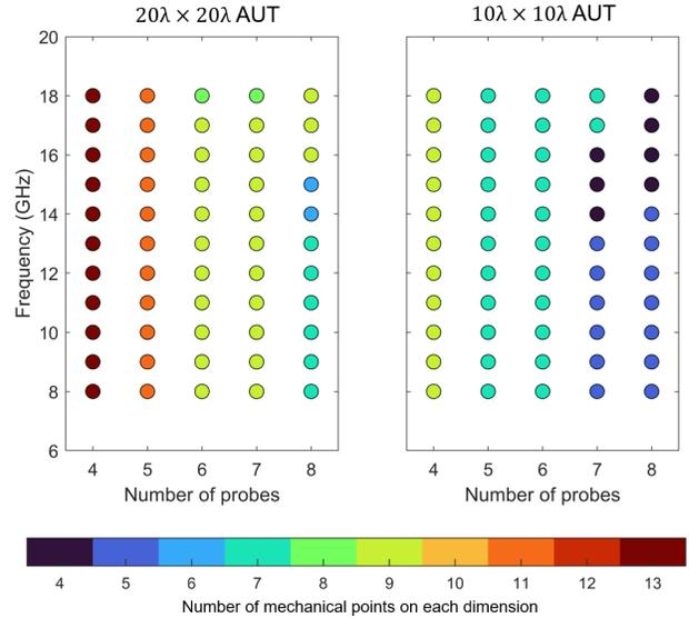
Fig. 4. Number of mechanical points of the PWM for several probe arrays.
