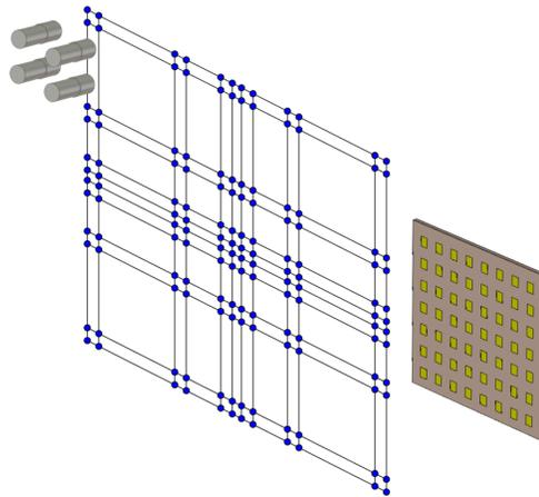
Fig. 1. Planar Wide Mesh measured by a  $2 \times 2$  probe array.
