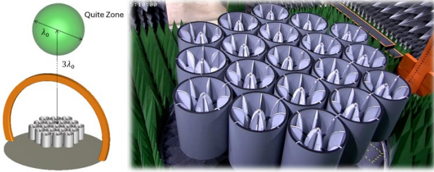
Fig. 1. Left: measurement scenario of the 19 element PWG array during validation measurement in the Pulsart by AGC spherical near field automotive range. Right: Image of the 19-element array during measurement.
