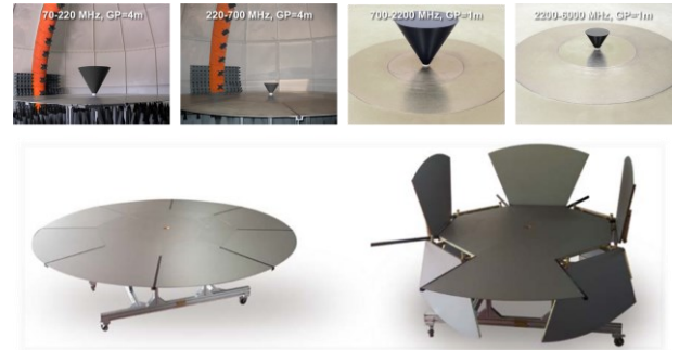
Fig. 2. Set of monocone antennas covering 70MHz to 6GHz, paired with geometrically scaled conductive ground planes.
