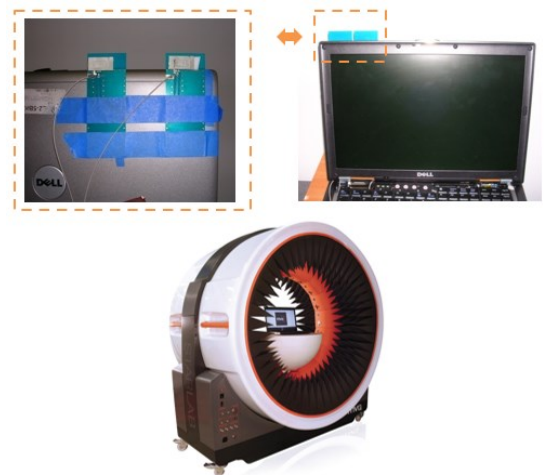
Figure 1: TIS test scenario with multiple antennas. Laptop with external antennas (left), antenna placement on the laptop lid (right), and SL18GHz spherical near-field measurement system used for accurate TIS determination (below).
