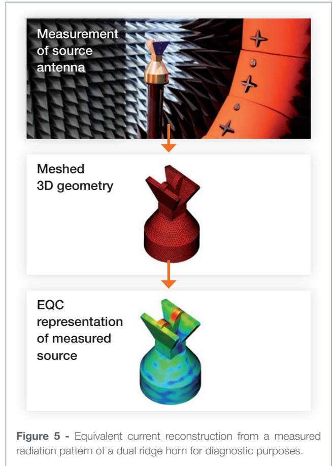
**Figure 5** - Equivalent current reconstruction from a measured radiation pattern of a dual ridge horn for diagnostic purposes.
