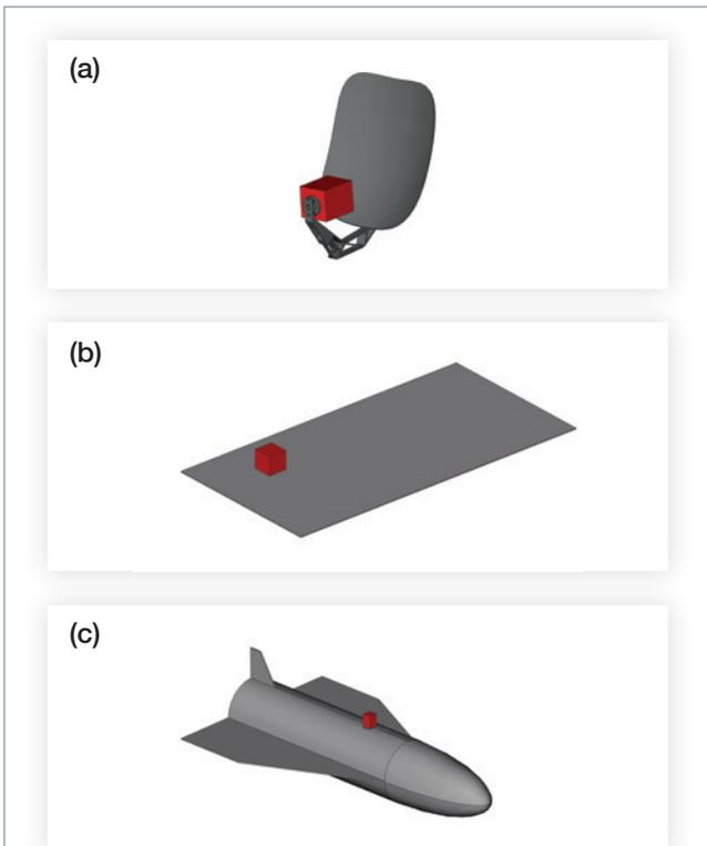
**Figure 9** - Test cases for the validation campaign of the Link between measurements and simulations. Reflector antenna fed by a horn (a); Flush mounted monocone antenna and open ended waveguide on a flat structure (b); Flush mounted monopole antenna on a curved structure (c). Equivalent Current representations appear as red boxes.
