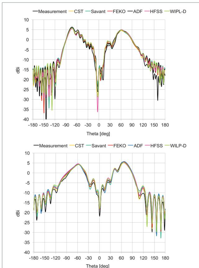
**Figure 14** - Directivity pattern of SMC2200 monocone antenna on rectangular plate @ 5.28 GHz;  $\phi=0^\circ$  plane (top),  $\phi=90^\circ$  plane (bottom). Measurement and simulation using measured source: CST [17], Savant [18], FEKO [19], HFSS [20], ADF [21], WIPL-D [22].
