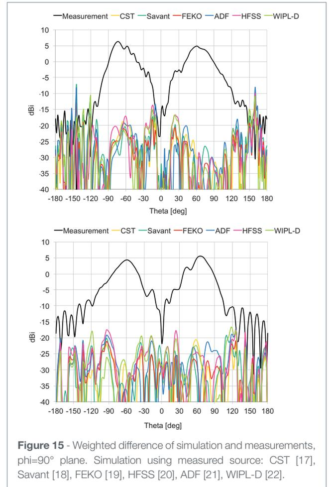
**Figure 15** - Weighted difference of simulation and measurements,  $\phi=90^\circ$  plane. Simulation using measured source: CST [17], Savant [18], FEKO [19], HFSS [20], ADF [21], WIPL-D [22].
