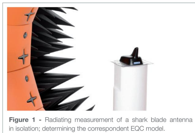
**Figure 1** - Radiating measurement of a shark blade antenna in isolation; determining the correspondent EQC model.
