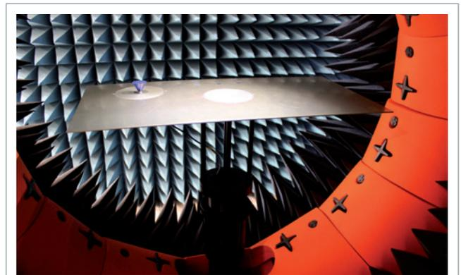
**Figure 10** - Rectangular ground plane validation structure - Measurement of SMC2200 monocone antenna in the MVG StarLab18 GHz.
