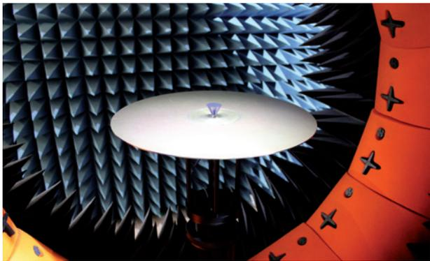
**Figure 11** - Measurement of the monocone antenna on a limited ground plane in the MVG, SL18GHz spherical near field multi probe system.
