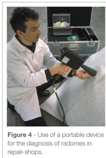
**Figure 4** - Use of a portable device for the diagnosis of radomes in repair-shops.
