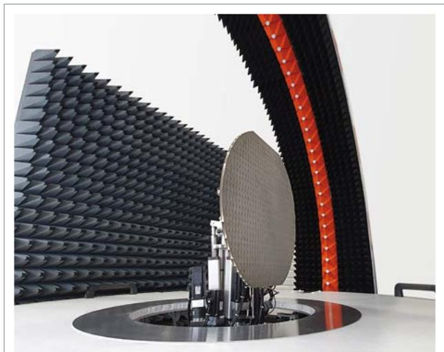
Figure 5 - Aerolab probe array and positioning system.
