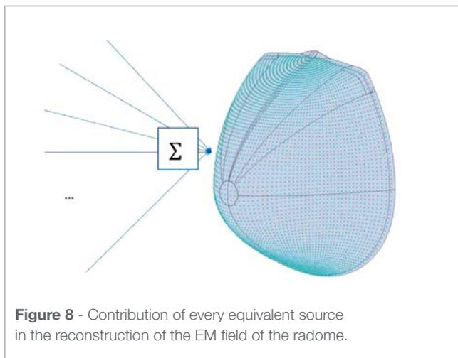
**Figure 8 -** Contribution of every equivalent source in the reconstruction of the EM field of the radome.
