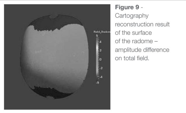
**Figure 9 -** Cartography reconstruction result of the surface of the radome – amplitude difference on total field.
