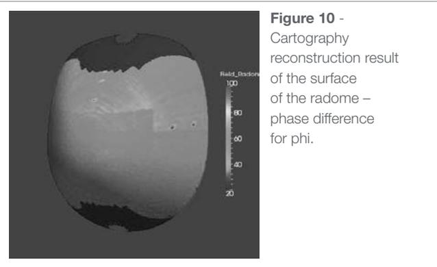
**Figure 10 -** Cartography reconstruction result of the surface of the radome – phase difference for phi.
