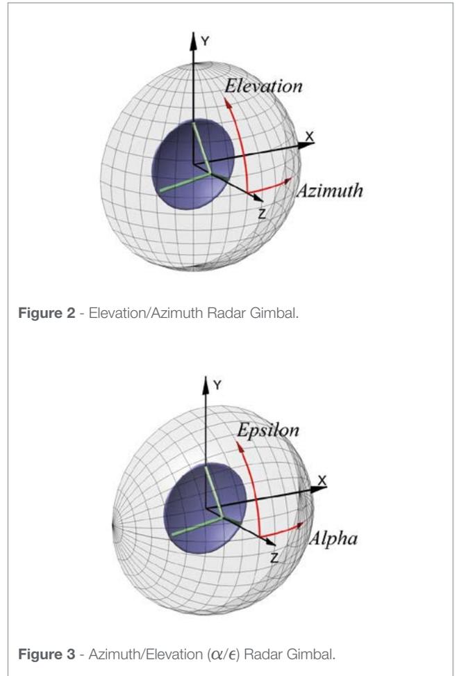
Figure 2 - Elevation/Azimuth Radar Gimbal.
